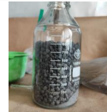
Raw materials – granules of hafnium dioxide
